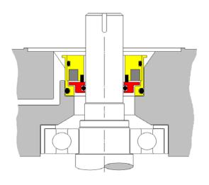
**ISOMAG** bearing seals eliminate the problems caused by leaking upper gearbox lip seals.
